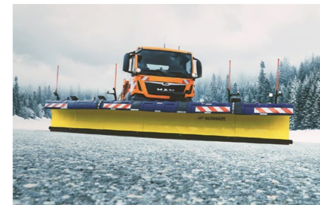
The Schmidt Tarron HP-2W snow plow has a working width of more than 20 feet at a 30° attack angle. (Picture above)
