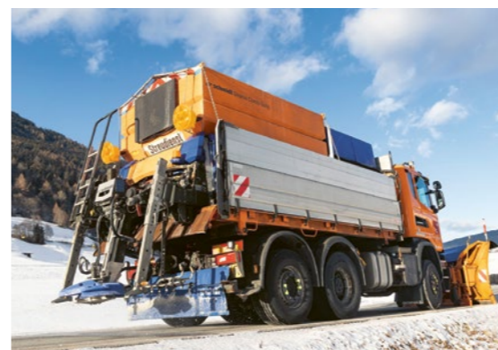
The Schmidt Stratos Combi Soliq allows the operator to apply different spreading materials using different methods, depending on the situation.
