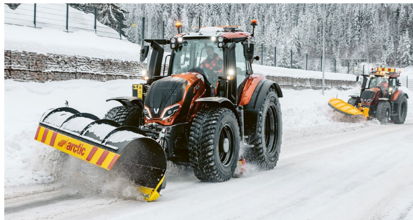
The Schmidt Tarron HP-2W snow plow has a working width of more than 20 feet at a 30° attack angle. (Picture above)
