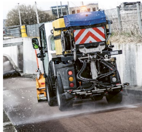
With the compact Nido CSP sprayer, icy roads and pathways can be treated efficiently and in an environmentally friendly way.
